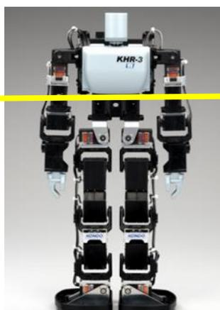
The arm of the dummy robot for Auto should be between the yellow line of KHR-3HV and the head. And wrap the specified KHR-3HV image around the dummy robot all the way up and down. In the case of Auto, do not attach the head
