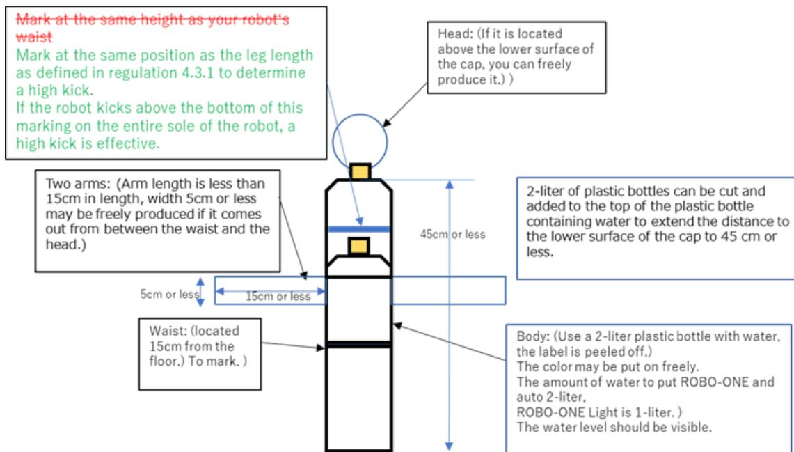
Figure 1 Dummy robot (other than auto)
